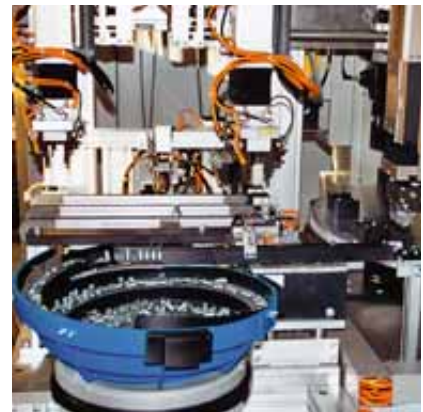
The optical fork and angle sensors are especially used for part monitoring in feeding technology and handling systems.
