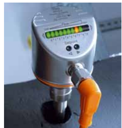
Evaluation system for local mounting.
