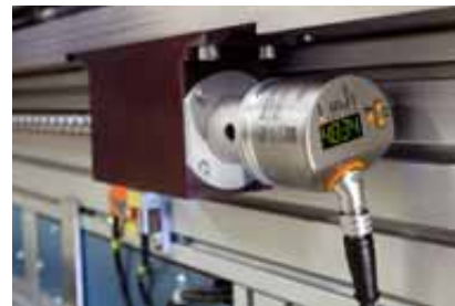
Spindle monitoring: encoder with display in the speed monitor mode.
